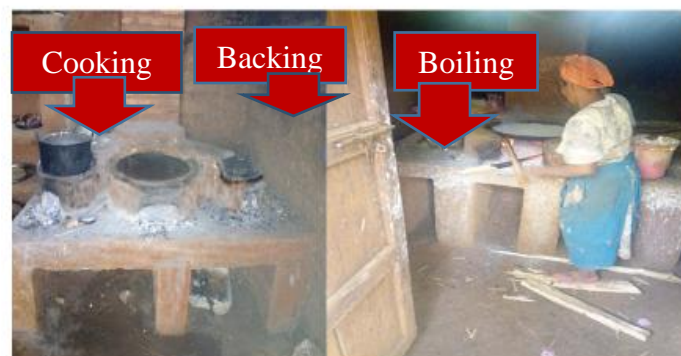
Figure 5. Improved multipurpose mud biomass cook stove. The stove tested in homes, known as the Multipurpose Mud Stove (Figure 3), is used for baking, cooking, and boiling. Constructed above ground from mud bricks and straw with an integrated chimney, it has three burning chambers: one for baking Injera and two for cooking other dishes like wot. The stove sits on a 180 cm × 150 cm smoke-free mud bed, 70 cm above the ground. The three stoves on the bed are connected by channels that allow smoke to burn fully before exiting through the chimney. The Injera stove is cylindrical, 25 cm tall and 60 cm in diameter, matching the mitad. The main stove is 40 cm in diameter and 23 cm high, while the secondary stove is 25 cm in diameter and 21 cm high. The chimney, built from mud bricks, reaches 150 cm, and each brick has a 16 cm × 14 cm central hole, made using two different molds.
