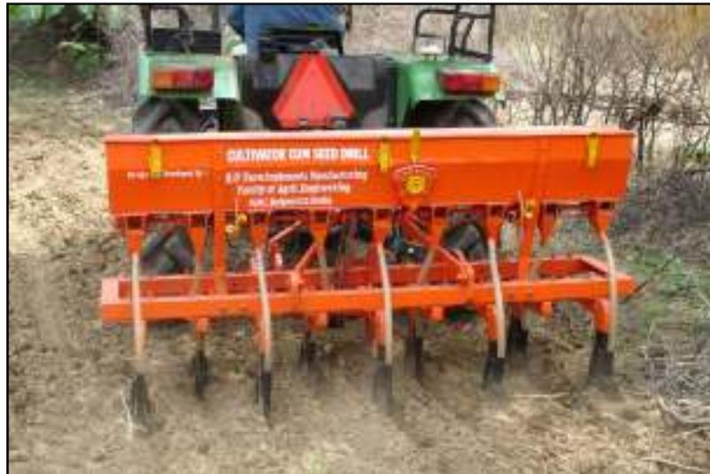
Figure 2: Field performance test for prototype cultivator
