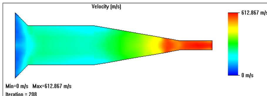
Figure 6: velocity analysis of circular nozzle
