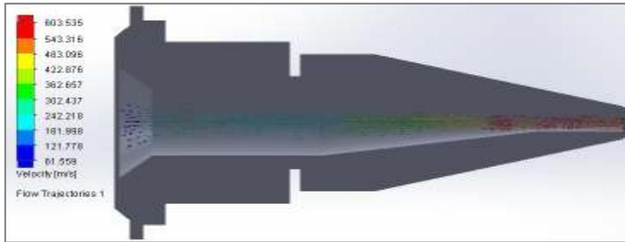
Figure 3: Velocity of circular nozzle
