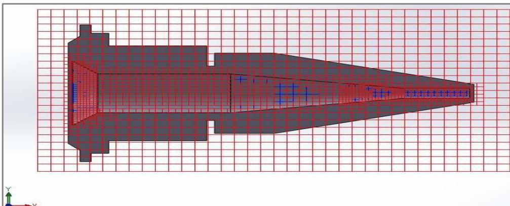
Figure 14: Meshing of Elliptical nozzle
