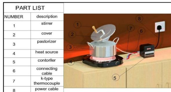
Figure 1: Pictorial view of experimental set-up
