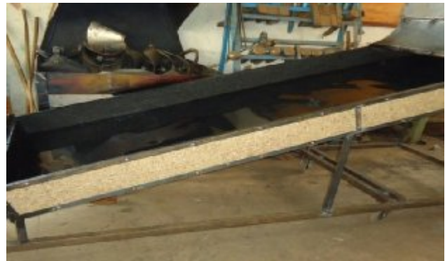
b) Solar collector after fabrication
