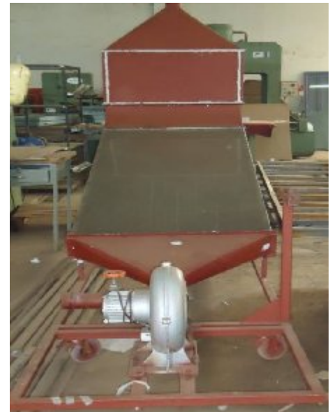
Fig.3: Constructed Solar Coffee Drying Machine
