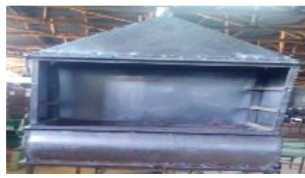
d) drying chamber during fabrication
