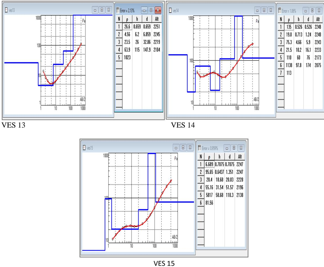
Figure 3 Interpreted Resistivity curves.
